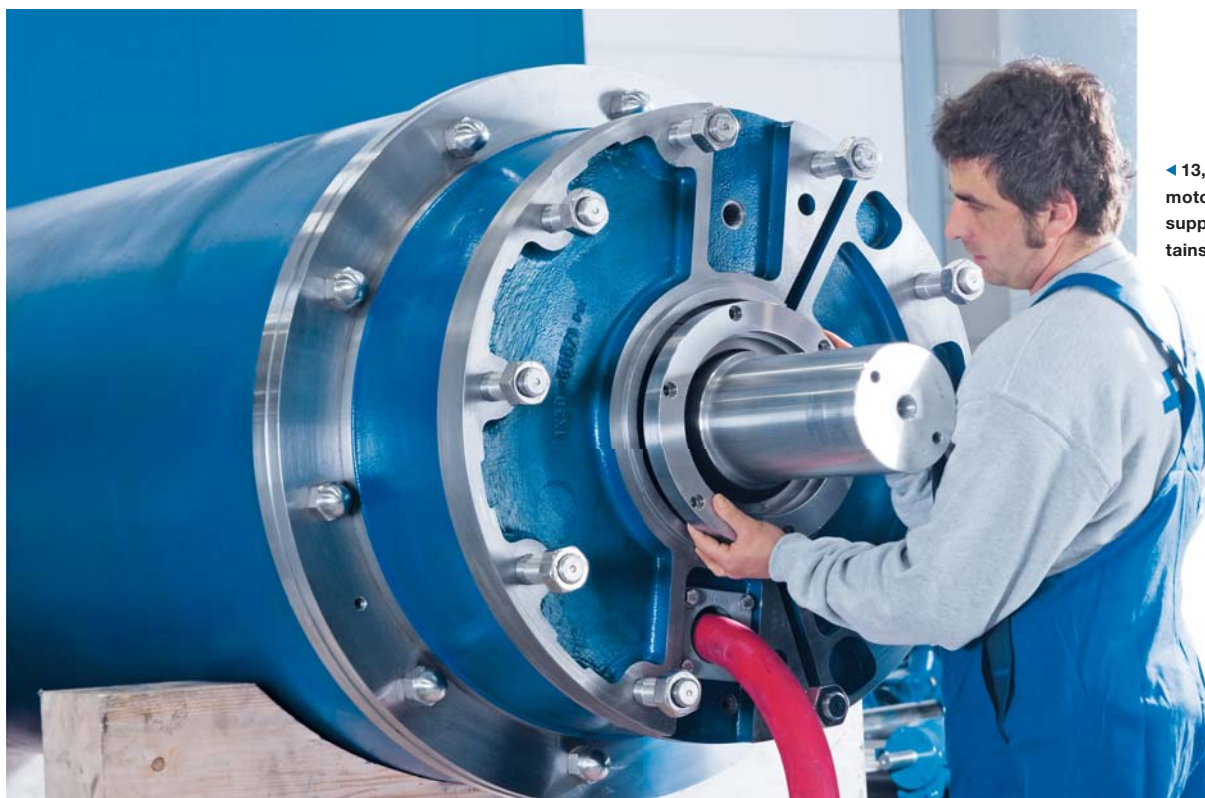
▲ Fitting four bottom intake pumps with ANDRITZ Ritz custom-made submersible motors in Marina Barrage, Singapore
