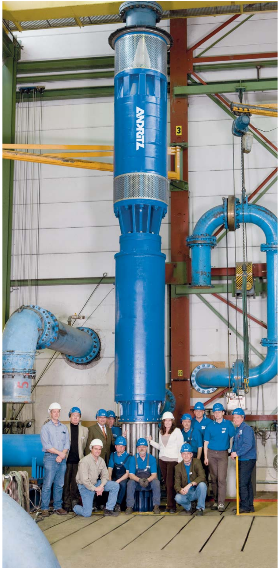
▲ View of a stator casing of a submersible motor
