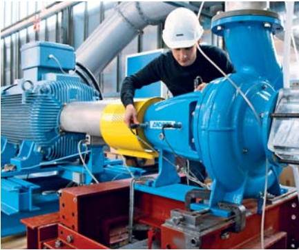
▲ Single-stage standard centrifugal pump on the test rig in Graz, Austria
