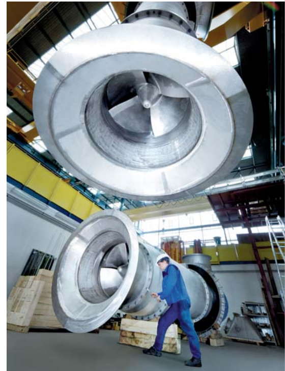
▲ Cooling water pumps for a power plant in Gent, Belgium
