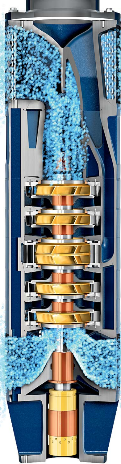
Flow simulation of the double suction HDM technology ▶
